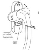
2. When the LED diode of the receiver flashes with a red light "the association button" should be pressed on the H-1 handle (located under the cover) and held pressed for at least 2 seconds. When the LED diode on the handle starts flashing with a red light we release the button.
