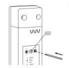
1. Signing out the H-1 handle from the receiver is initiated by pressing the right signing out button (red triangle - ▲ ) on the receiver and pressing it for at least 2 seconds until the LED diode starts flashing with a red light, then we release the button.
